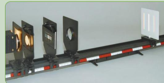
Experiment P 37 21 | Diffraction by Grating
