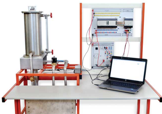
Level process control experiment (PLC, frame and Laptop not included).
