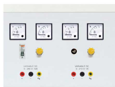
Variable DC output of 0-240 VDC and 0-240 VDC are equipped with panel meter and current limiter of fuse.
